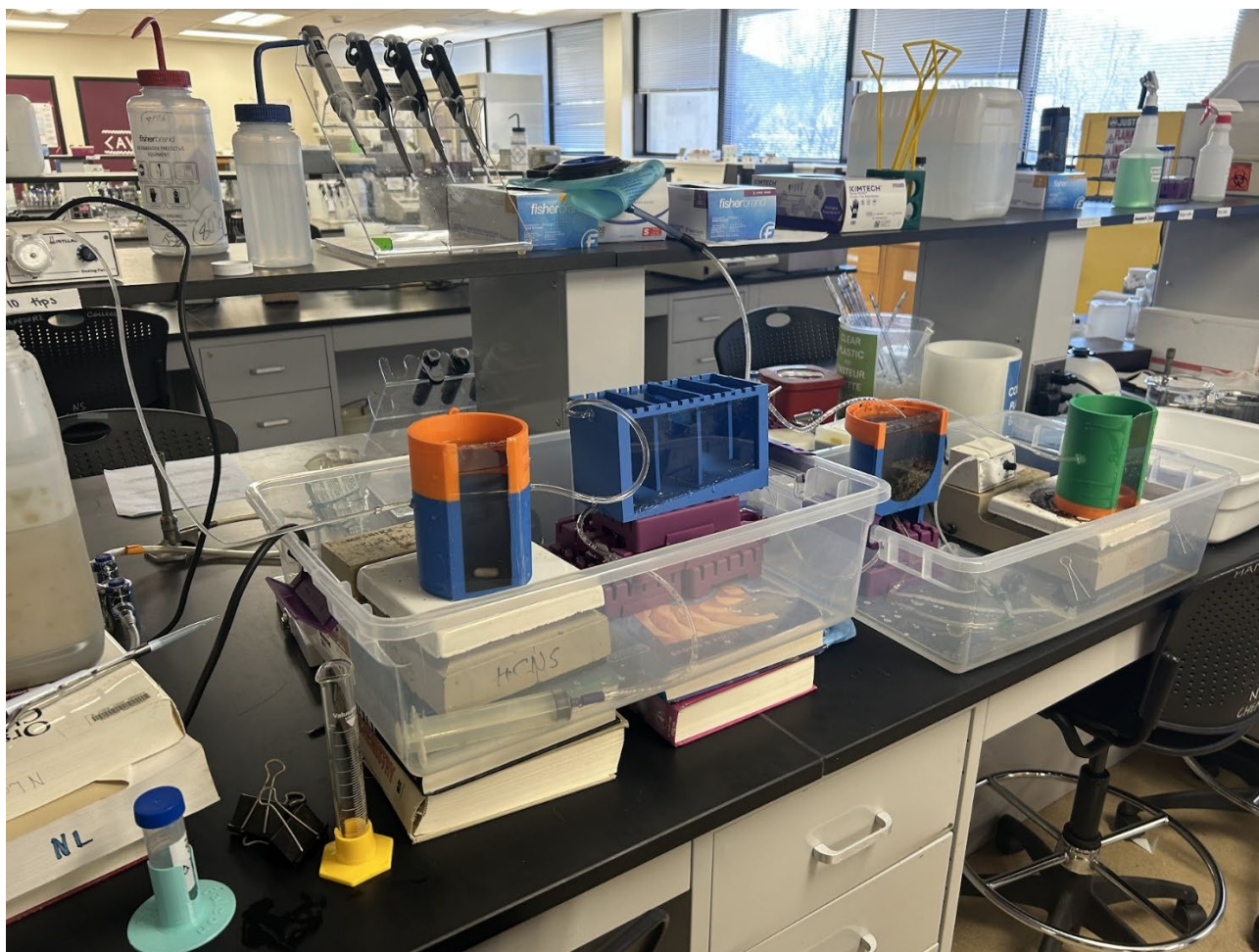
Figure 1 Photo of the assembled drinking water treatment plant where untreated water (leftmost bottle, moving to the right) is pumped into the coagulant dosing basin before entering the sedimentation basin. The filtration basin was filled with sand a granular activated carbon before a final dosing basin for disinfection.
