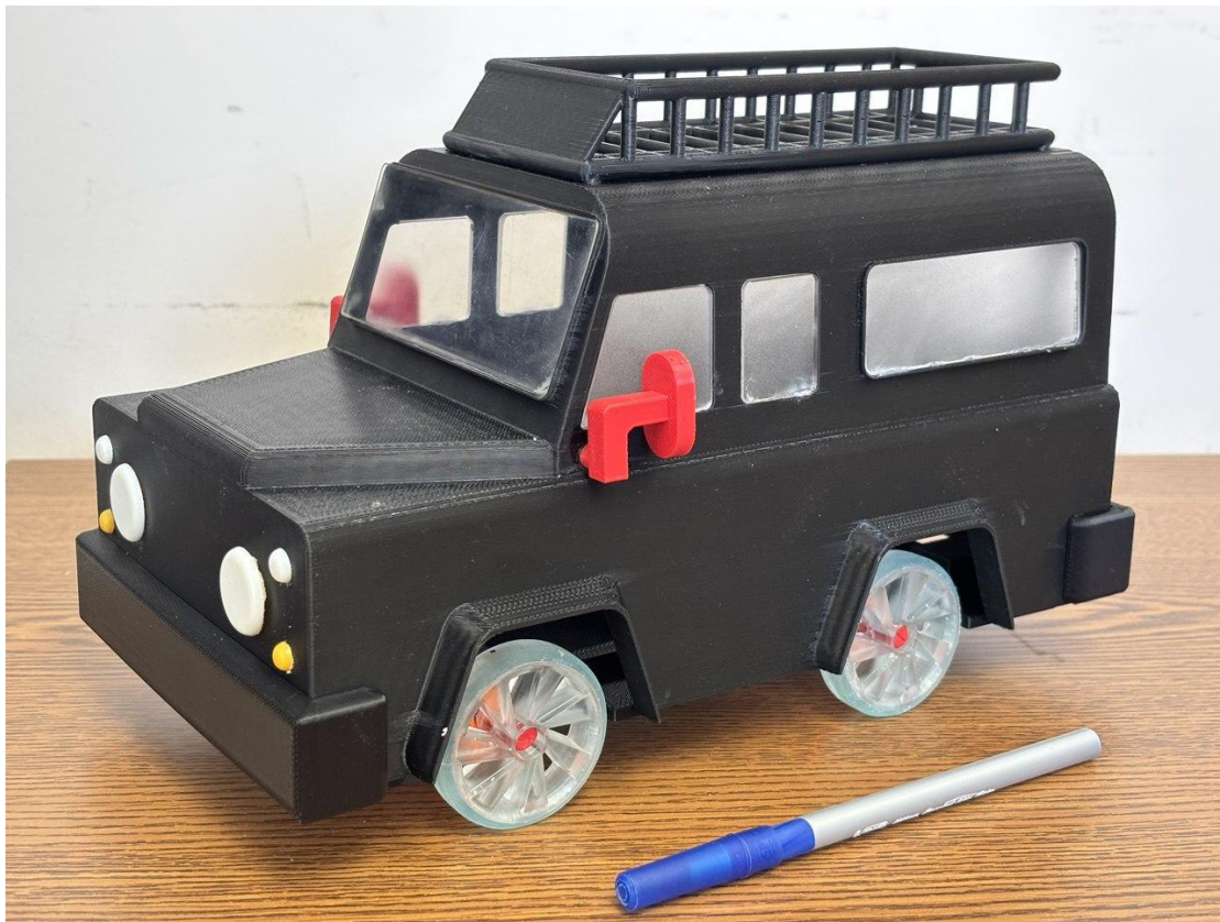
Figure 2. Representation of the 3d printed and assembled car parts.
