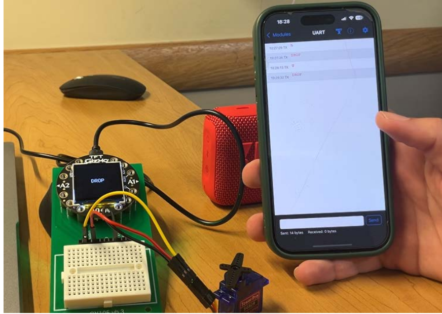
Figure 4: Student-built CPS demonstrating Bluetooth activation of servo motor.
