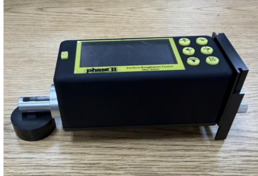
Figure 2. Experimental setup for stylus-based surface roughness measurements.
