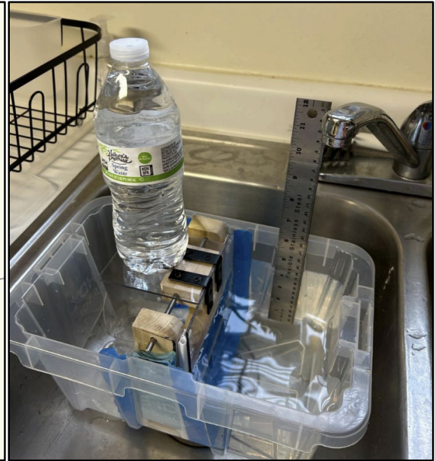
Figure 7.a: Sketch design for hydrostatic gate Figure 7.b: Hydrostatic gate setup with water bottle as a variable weight
