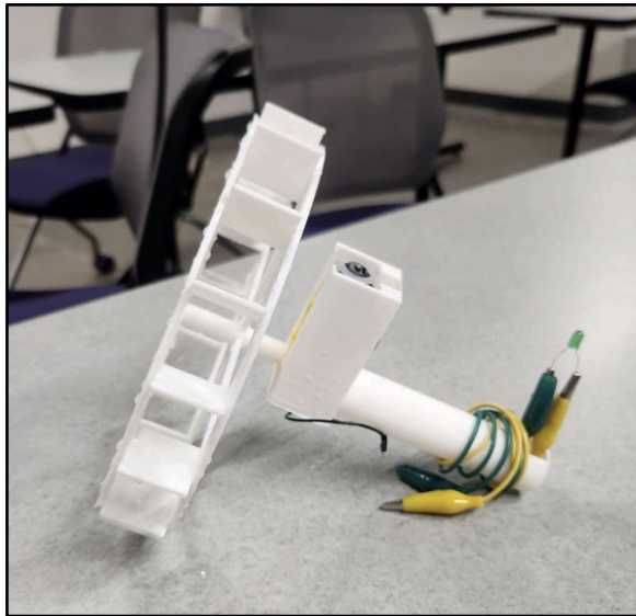
Figure 8.a: Water wheel desing with gearbox and LED attachment
