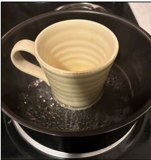
Figure 4.a: Heating of test liquid in mug using boiling water
