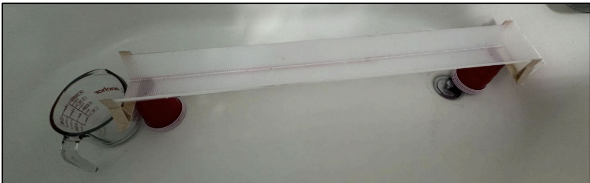
Figure 6.a: Trapezoidal channel set up in tub at specified slope
