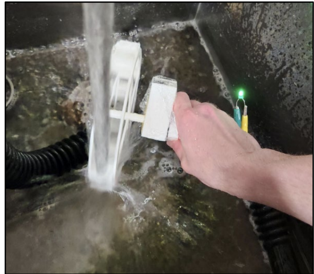
Figure 8.b: Operating water wheel lighting LED
