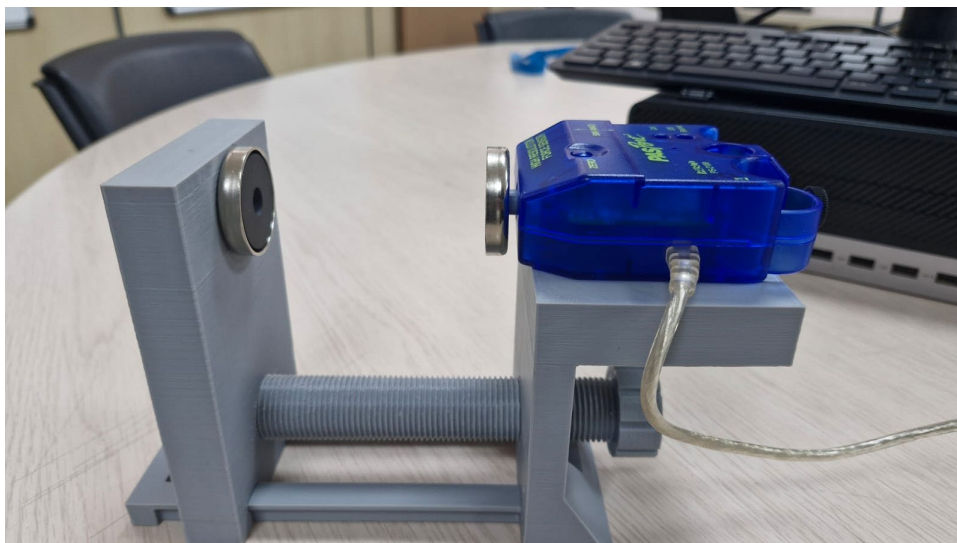
Figure 3. Initial apparatus setup with encapsulated magnets and bottom-mounted screw-based distance adjustment (authors' work).
