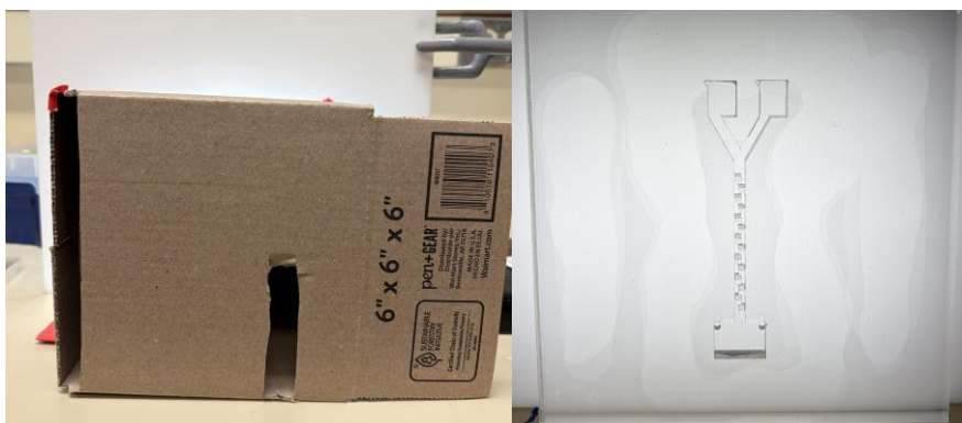
Figure 1. Left: Cardboard frame used for light isolation. Right: Main Module with y-shaped chamber and offset reservoirs for on demand mixing.
