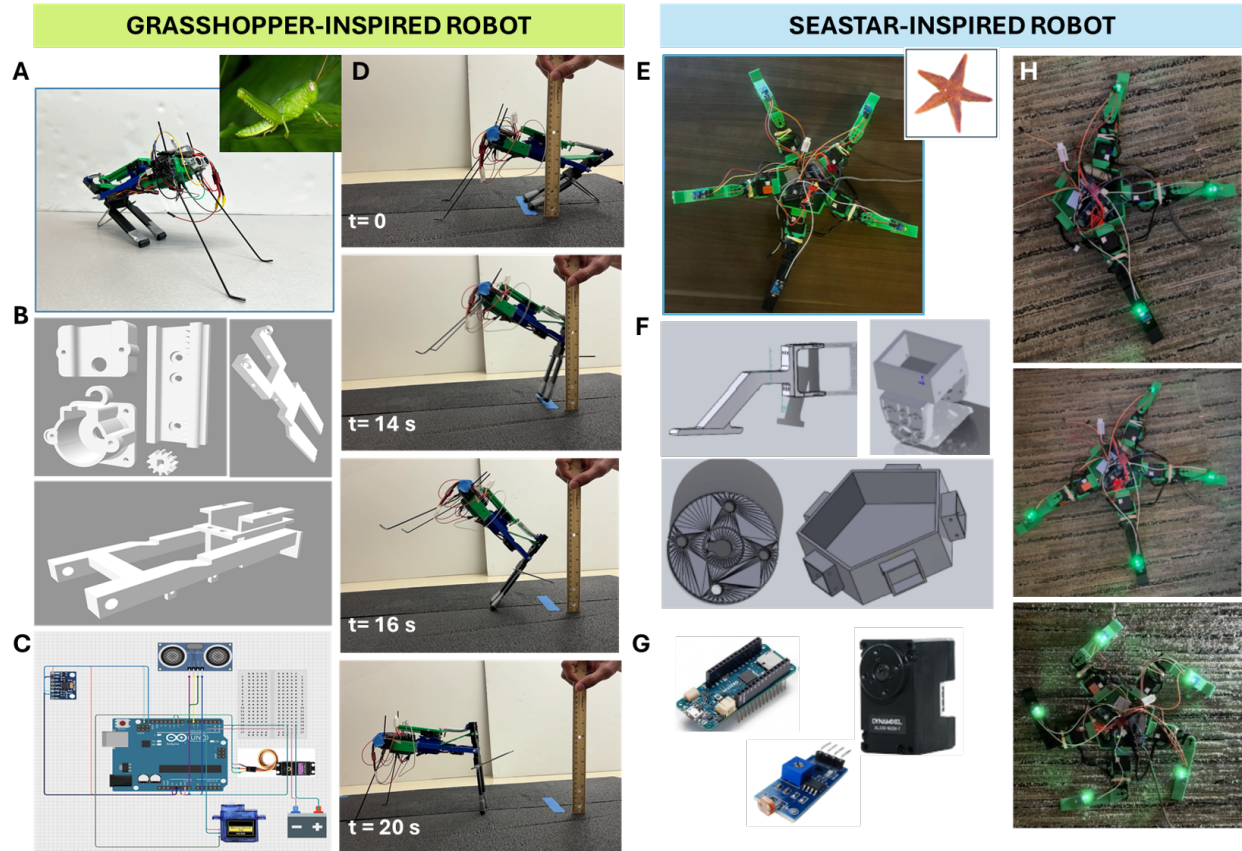
Figure 3: Example student projects from the Experimental Robotics course. (A–D) Grasshopper-inspired Robot. (A) final physical prototype; (B) CAD assembly of the mechanical components designed in SolidWorks, highlighting the spring-loaded catapult mechanism; (C) circuit schematic of the electronic control system; and (D) snapshots of experimental trials evaluating jumping performance on a foam surface. (E–H) Seastar-inspired radially symmetric robot: (E) final physical prototype; (F) CAD model detailing the modular dual-servo revolute joints and central body; (G) electronic sensing, actuation, and control units; and (H) experimental gait analysis demonstrating mobility across various limb configurations (three, four, and five legs). The names of the students who completed the projects are listed in the Acknowledgments section.
