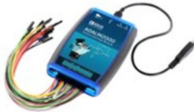
Figure 1. The ADALM2000 (M2K) active learning module
