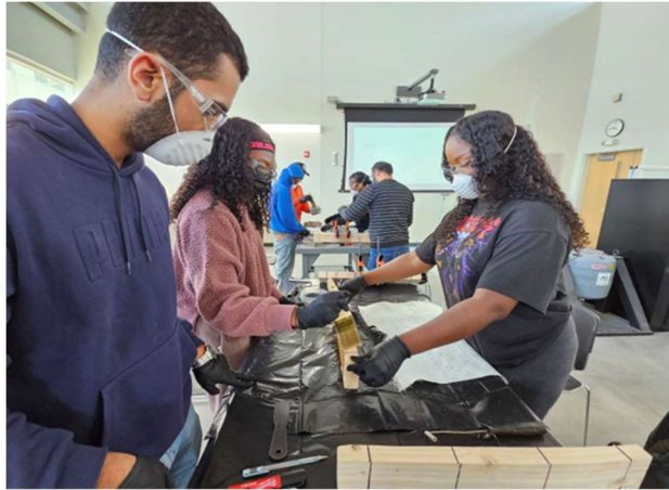
Figure 9. Partial wrapping of GFRP on timber beams by students
