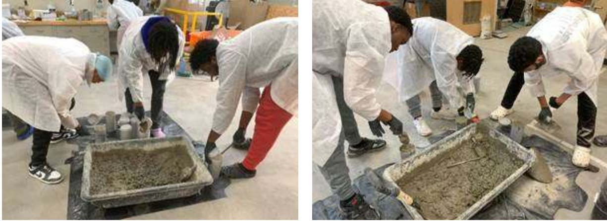
Figure 12. Casting of concrete cylinders by student groups.
