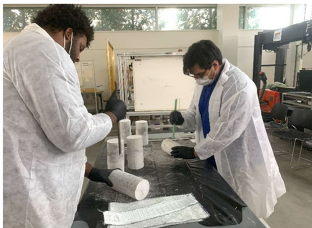
Figure 13. Surface preparation before GFRP application
