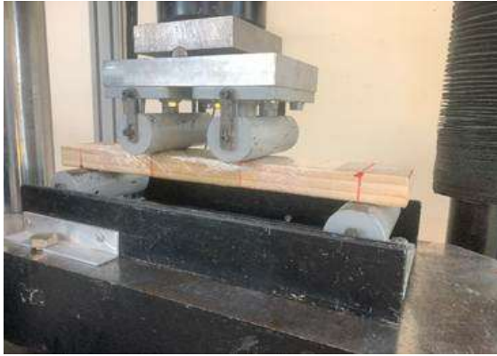
Figure 11. Flexural strength test on a partially wrapped timber beam.
