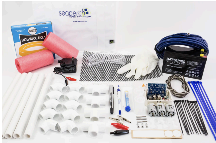
Figure 3: The SeaPerch ROV kit includes PVC frame components, buoyancy materials, a CAT 5 tether cable and butyl rubber tape, and core wiring and safety items. In addition, the kit provides dedicated packs for the controller (PCB, switches, fuse holder and RJ45 jack), thrusters, and propellers.
