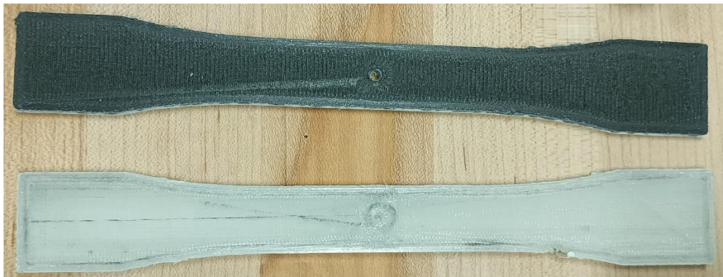
Figure 6: Surface irregularities observed in AM specimens
