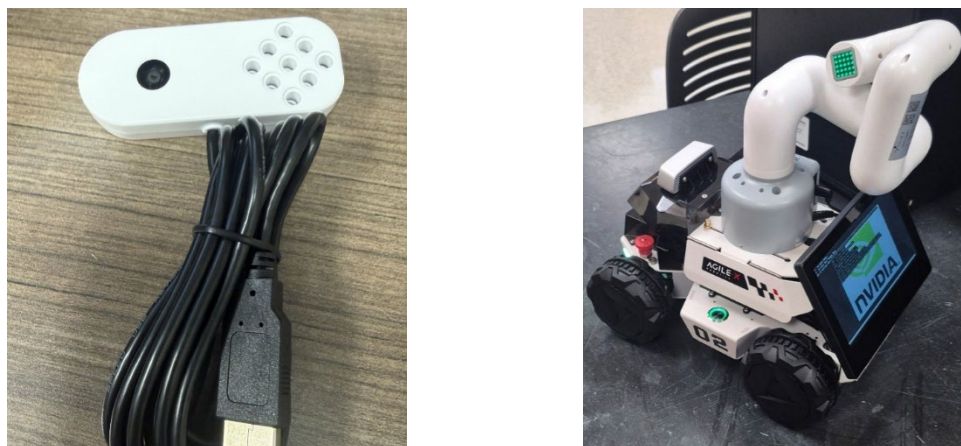
Figure 7 Camera Flange for the Mycobot 280 mounted on top of a LIMO Cobot
