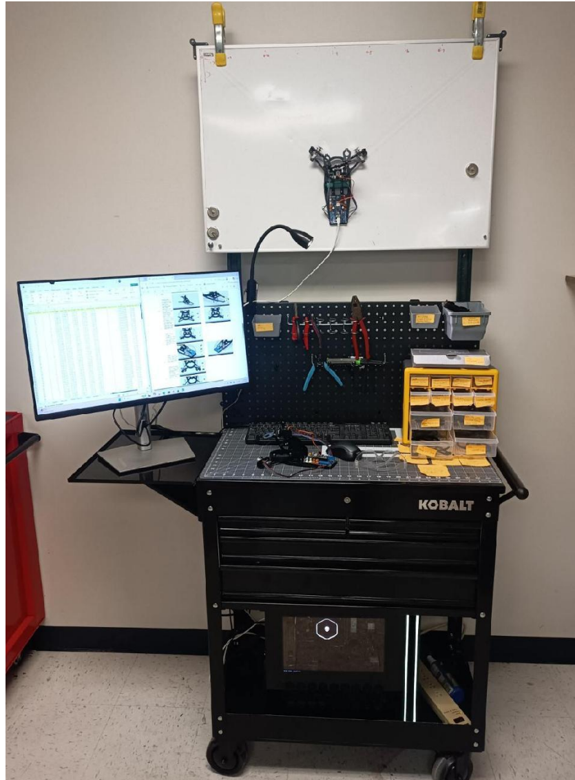
Figure 2: Manufacturing assembly cell for drawing robot
