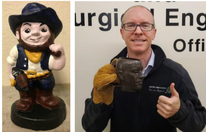
Fig. 1. (a) A slip casted model of the school mascot "Grubby". (b) Ceramic slip casted product from a 3D scan of the Metallurgical Engineering Departments Head.
