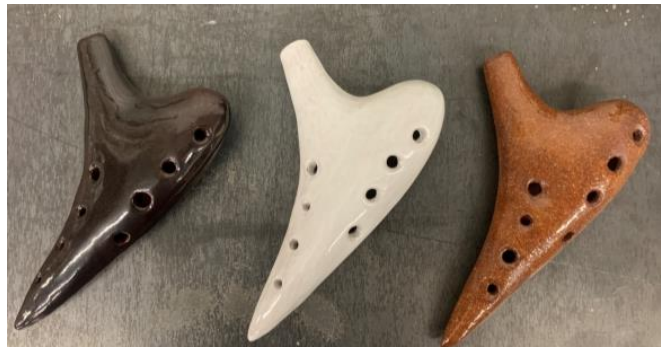
Fig. 2. Three perfectly tuned ocarinas capable of playing Twinkle Twinkle Little Star were made from 100% Black Hills minerals.
