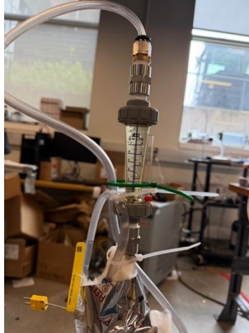
Figure 4. The flowmeter is connected using fittings sealed with Teflon tape. The flowmeter that is used to measure the flow of water through the helical copper coil. Water flows upward through the flowmeter, and flow rate should be read at the bottom plate location.
