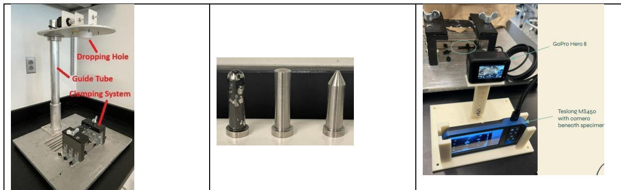
Figure 5: a) Impact Tester, b) Strikers, and c) Video Recording Systems with Two Cameras [14]
