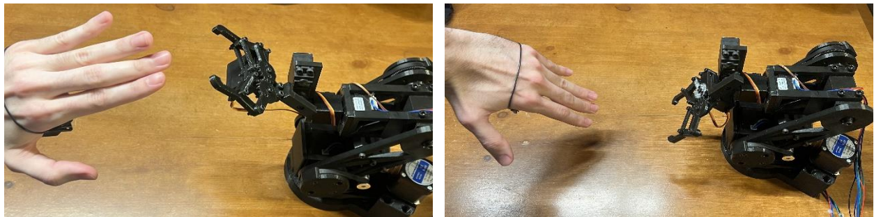
Figure 11. When tilting the wearable module up, the robot's wrist also moves up (left). When tilting the wearable module down, the robot's wrist also moves down (right)
