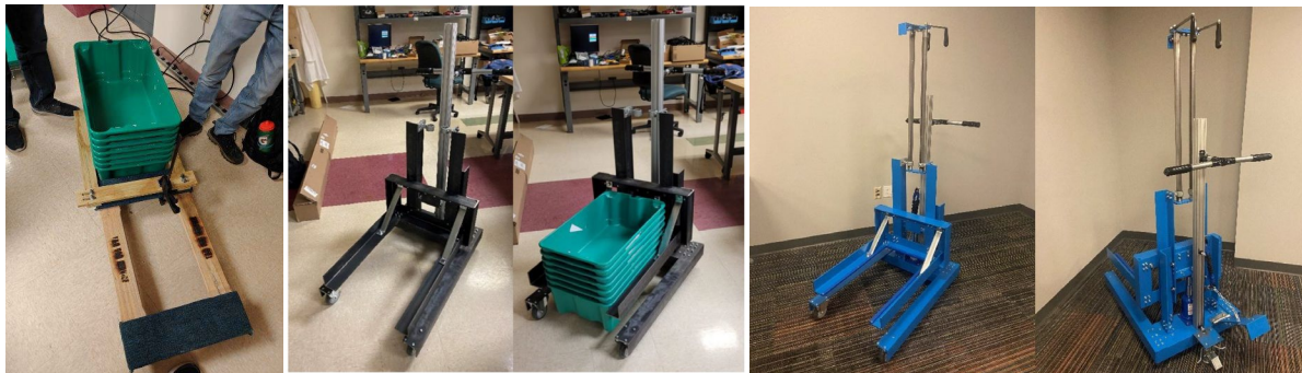
Figure 6. Fork-Dolly Test Assembly (Left) 1 st Prototype (Middle) Final Prototype (Right)
