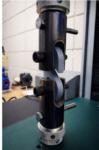
Figure 3 Tensile testing configuration used to evaluate additively manufactured hook specimens under static loading.
