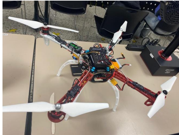
Figure 8. Quadrotor assembly and calibration developed at Tecnológico de Monterrey.
