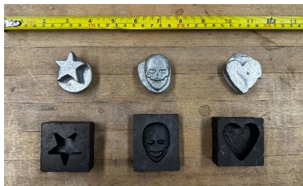
Figure 2. The graphite molds and their associated casted aluminum parts. Students could choose which mold to use, and they had the opportunity to cast twice.
