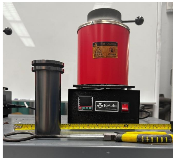
Figure 1. The aluminum melting furnace with the associated graphite crucible and tongs to lift the crucible.
