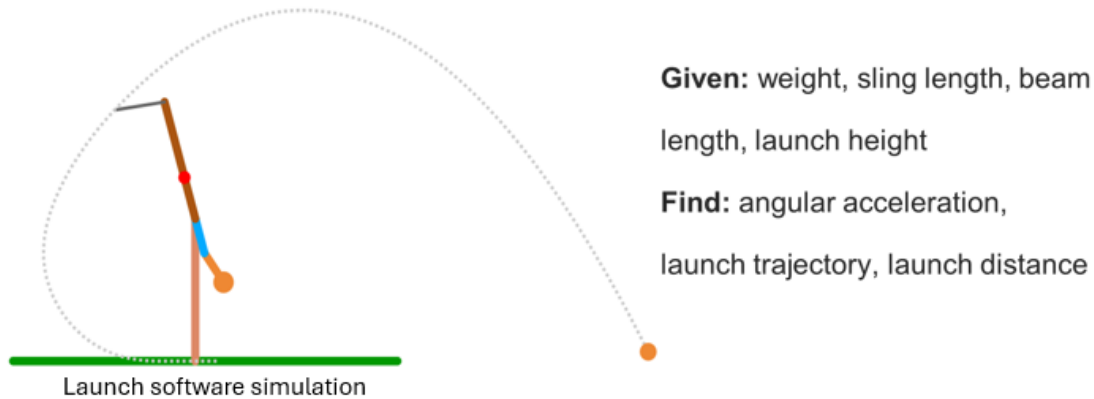
Figure 4: Schematic of trebuchet demonstration for Dynamics.
