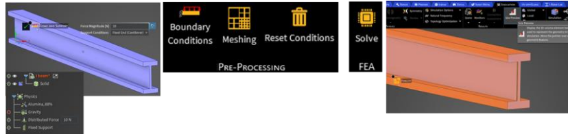
Figure 3: Pre-Processing & FEA (Solving)
