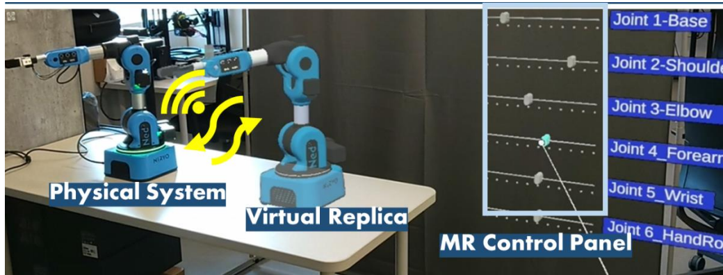
Figure 6. The synchronization between the physical Niryo Ned2 robotic arm and its virtual replica in the proof-of-concept XR-enabled teleoperation platform.
