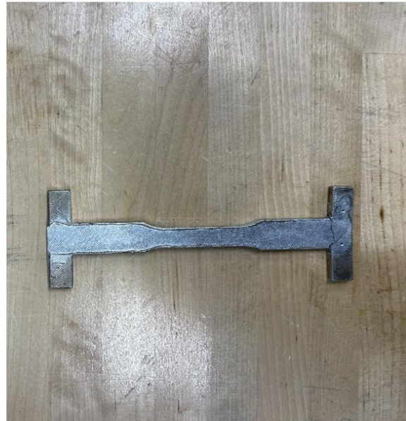
The figures about show the finished sand mold prior to removing the pattern, and a cast specimen after being cut from the casting.
