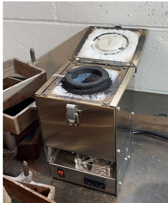
The figure on the left shows aluminum pieces being measured out for casting, and on the right is the benchtop casting furnace.
