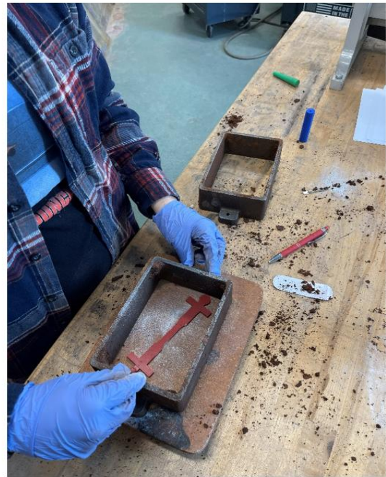
Students produced sand molds for tensile specimens using 3D printed patterns.
