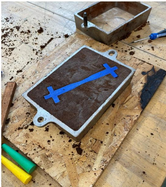
The figures about show the finished sand mold prior to removing the pattern, and a cast specimen after being cut from the casting.
