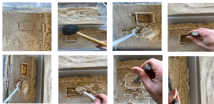
Figure 2. Demonstration of the construction of shallow foundation
