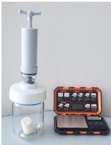
Figure 1. Experimental setup for students consists of marshmallow, handpump vacuum chamber with vacuum sealed lid, calipers, and electronic scale.
