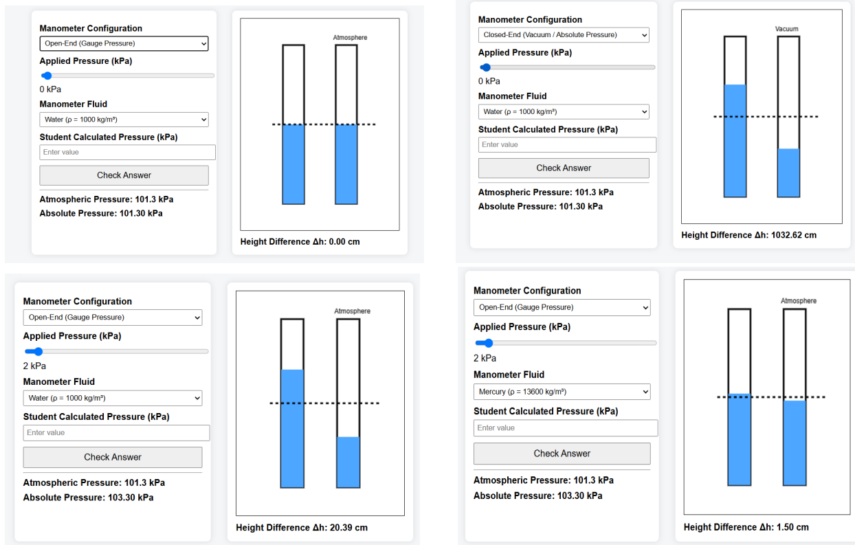
Figure 16: Screenshots of Lab Simulation about using manometers and measuring pressure
