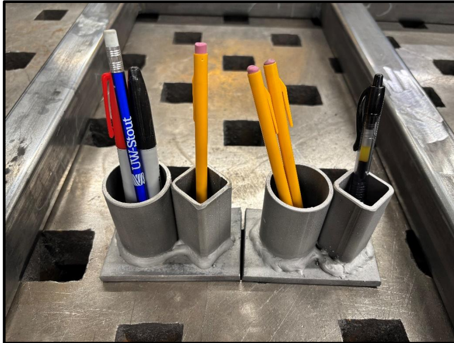
Fig. 4. Pencil holder weldment completed by the Yaskawa welding robot (left) and completed manually by a student (right)
