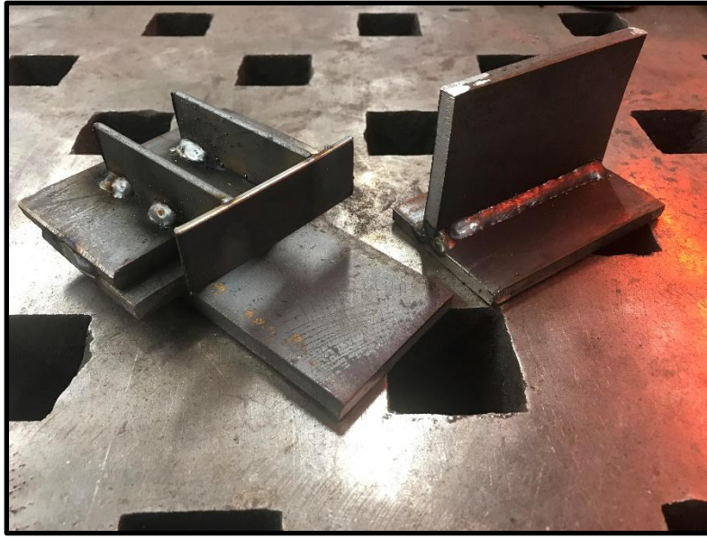
Fig. 3. The T-Joint weldment used in the semester 2 demonstration (right) and the fixture used to tack the members together (left) [13].
