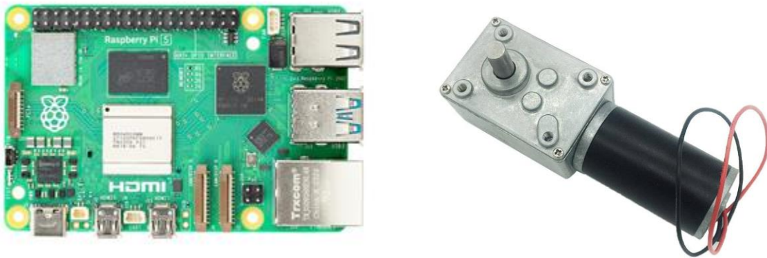
Figure 2. The Raspberry Pi 5 unit and the 12V DC Motor utilized in the project
