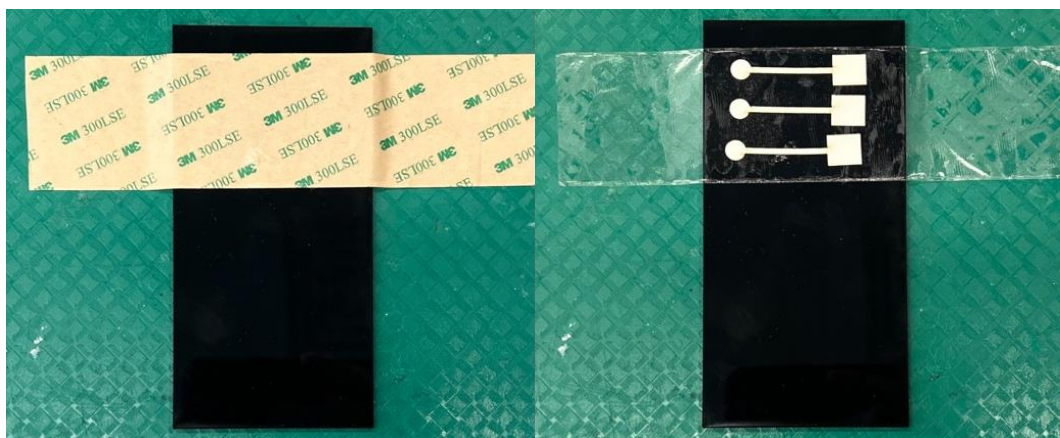
Figure 3: Photos from manual that show how students are to adhere their paper channels to the acrylic slab
