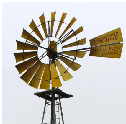
Figure 11: Farm windmill achieves zero steady state error for wind speed and direction naturally
