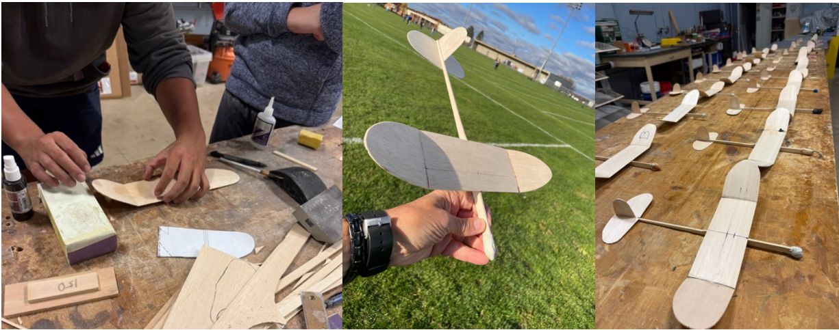
Fig. 2. (Left) Students shaping the wings for their Flips. (Center) A completed Flip ready for testing. (Right) Small variations in sanding, alignment, and assembly can be seen in the Flips despite following the same plans.
