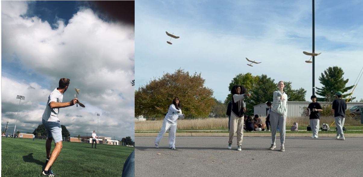
Fig. 3. Hand-launch testing enabled immediate observation of pitch, stability, and glide performance, allowing rapid iteration within minutes.
