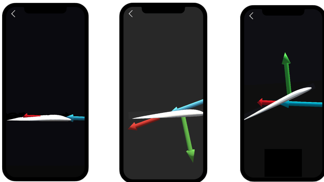
Figure 1. AR Scene showing how the velocity (blue), drag (red) and lift (green) vectors change with angle of attack.
