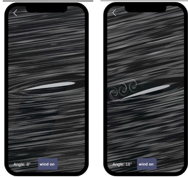
Figure 3. (a) Airfoil through the airmass below the critical angle with the air flowing around the airfoil. (b) At and above the critical angle, the air mass becomes turbulent as shown by the vortices at the lower left edge of the airfoil.
