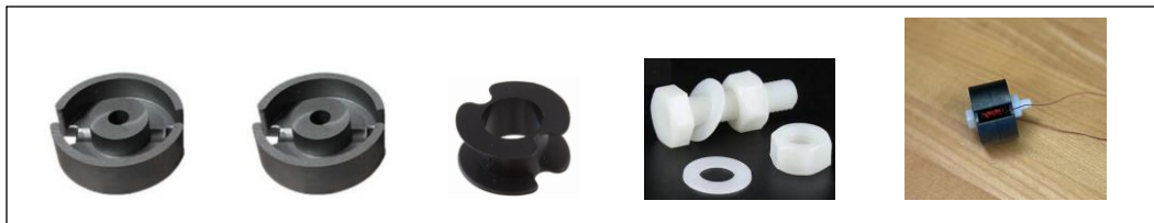
Figure 7. Components used to build the inductor and the assembled inductor.
