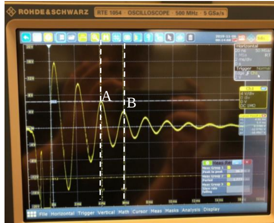
Figure 3. A damped sinusoidal waveform was generated by the piezoelectric strip oscillation and captured by the oscilloscope.
