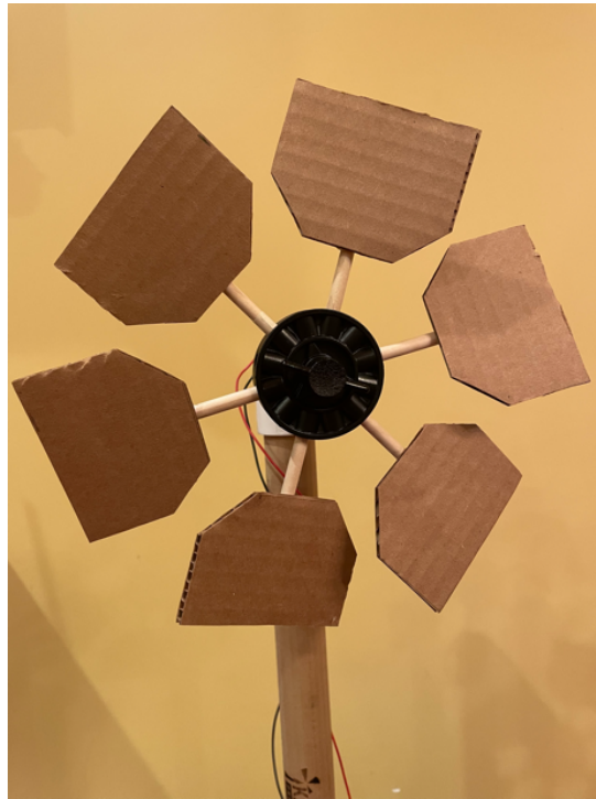
Figure 2. Image of Team AJEs Ago Design 1 Wind Turbine Blade System
