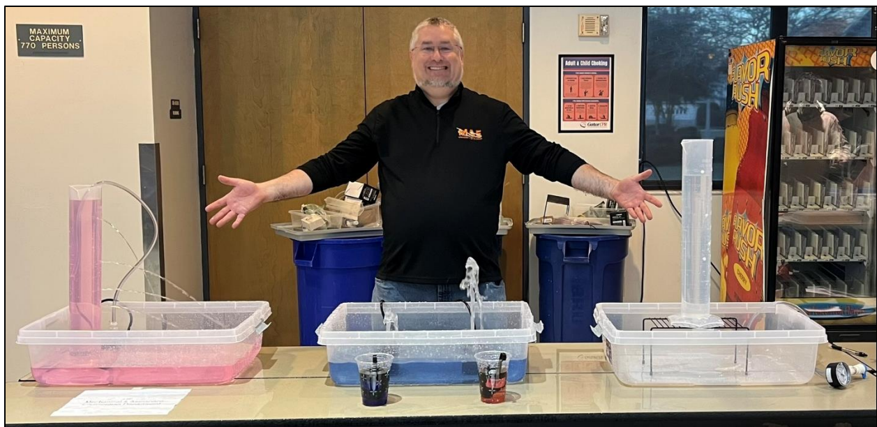
Figure 1: Educational fluids kits illustrating (Left) horizontal jets with flowrates metered by vena contracta, (Center) vertical free jets using an aquarium pump, (Right) hydrostatic pressure, and (Front) viscosity.
