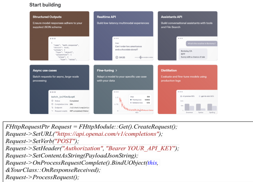
Figure 4: Integration of the OpenAI API into the Unreal Engine–based plugin, enabling narrative task interpretation while preserving deterministic and constraint-aware execution.
