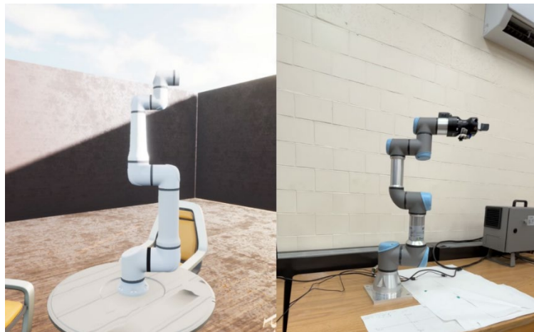
Figure 5: Pilot implementation of the narrative-driven digital twin framework, showing the Unreal Engine–based UR3e simulation (left) and the corresponding physical UR3e robot (right).
