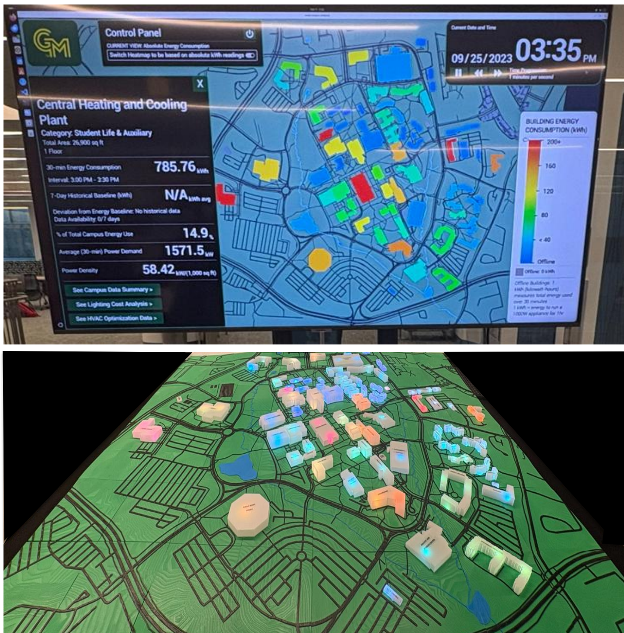
Figure 1. Integrated digital and physical 3D campus energy visualization system
