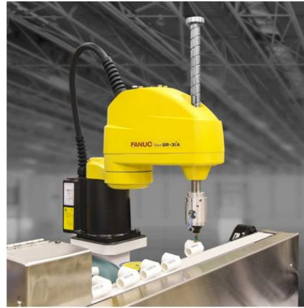
Figure 1: (A) A two-DOF robot manipulator. Motor 1 rotates L_1 , and motor 2 rotates L_2 relative to L_1 . (B) A real-world SCARA robot performing a pick and place operation.
