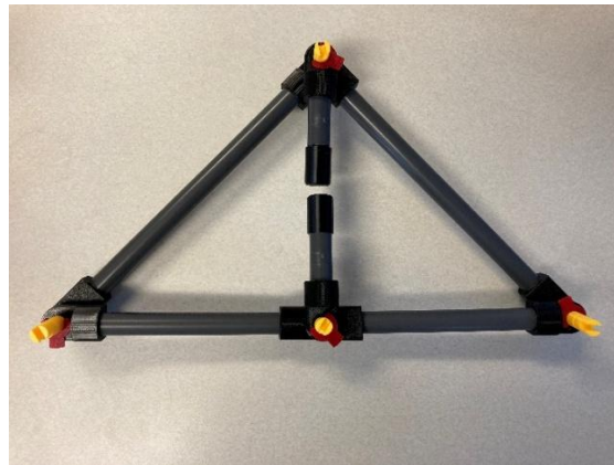
Figure 2. Truss showing the internal cut
