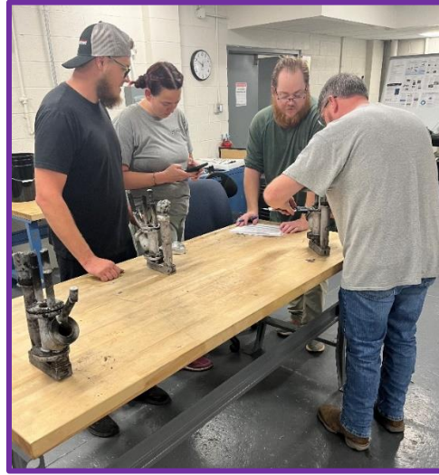
Figure 7. Bootcamp participants are measuring the finish quality of the cast part in terms of dimensional accuracy and surface roughness
