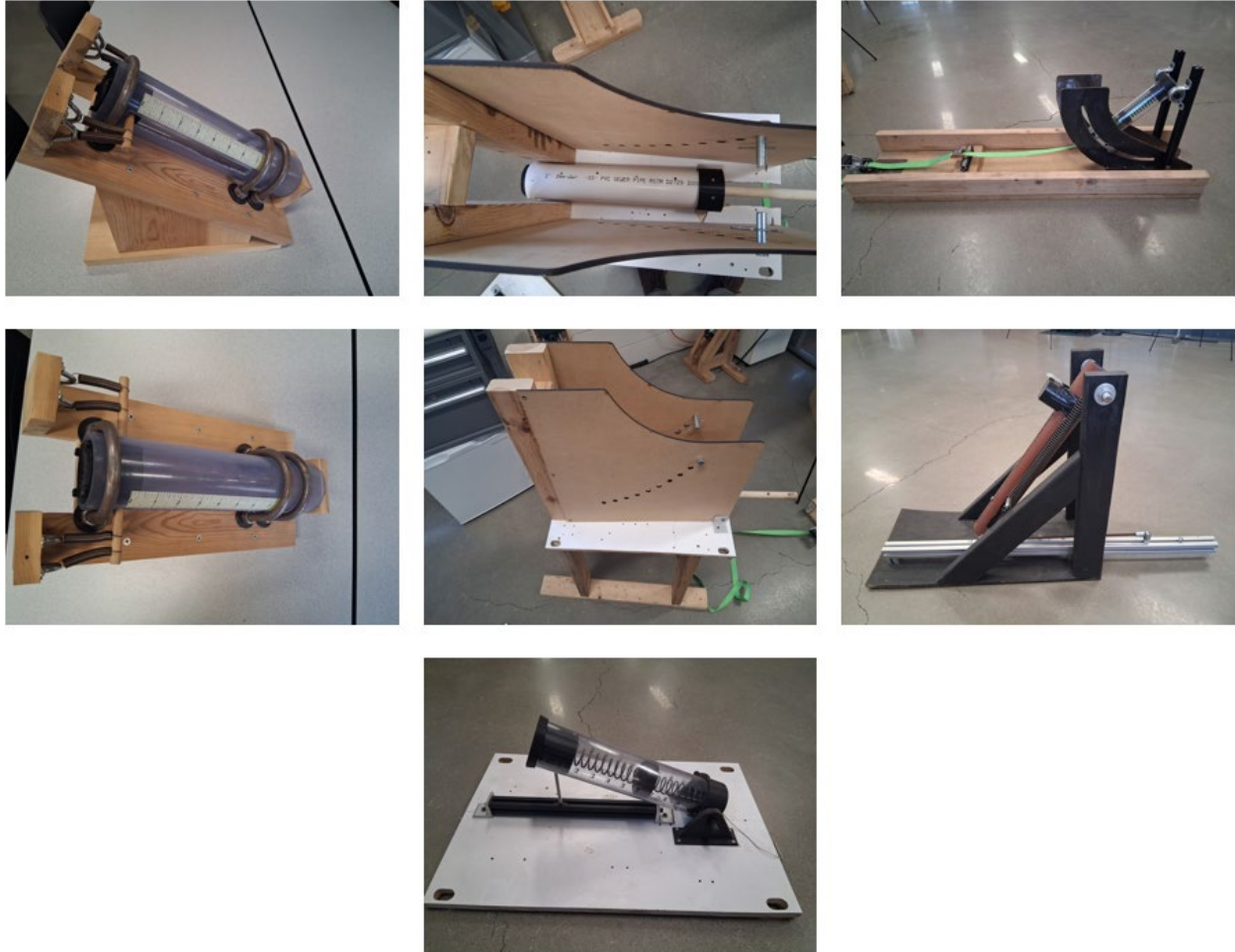
Figure 1: Representative launcher builds from students. Left column is two views of the same launcher using extension springs and a fixed launch angle. Middle column top two photos are same launcher using a compression spring and very thin PVC for a barrel with variable launch angles. Center bottom is a launcher using a clear barrel with compression springs in series and a variable launch angle. Right top is a robust design using a compression spring, variable launch angle, and a ratchet strap with release to fire while right bottom is similar but uses an extension spring and has a makeshift sight but no release mechanism.
