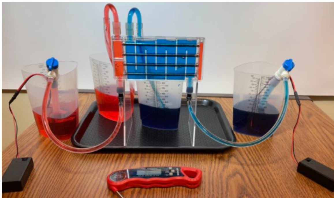
Figure 2. Shell and tube heat exchanger LCDLM.
