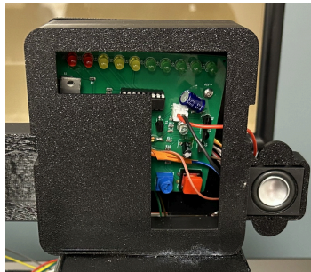
Figure 6. Final Stage LED Indicator and Integrated Speaker
