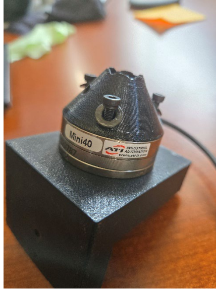
Figure 4: ATI Mini40 load cell shown with semi-traversable test stand head and sting holding assembly.
