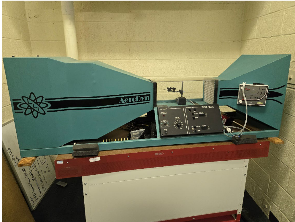
Figure 1: Derelict Learning Labs Inc. Aerodyn low-speed instructional wind tunnel shown before retrofit.
