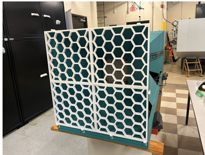
Figure 6: Learning Labs Inc. Aerodyn wind tunnel shown with 3D printed (PLA) honeycomb inlet grate.
