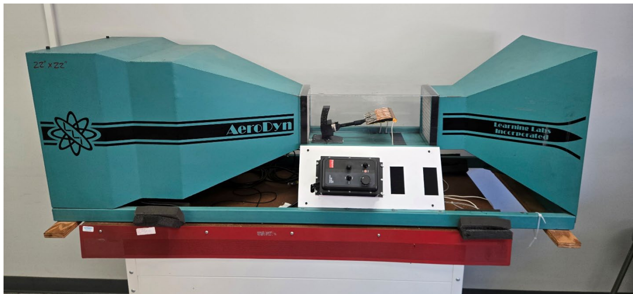
Figure 7: Learning Labs Inc. Aerodyn wind tunnel shown with small-scale airfoil model after retrofit.
