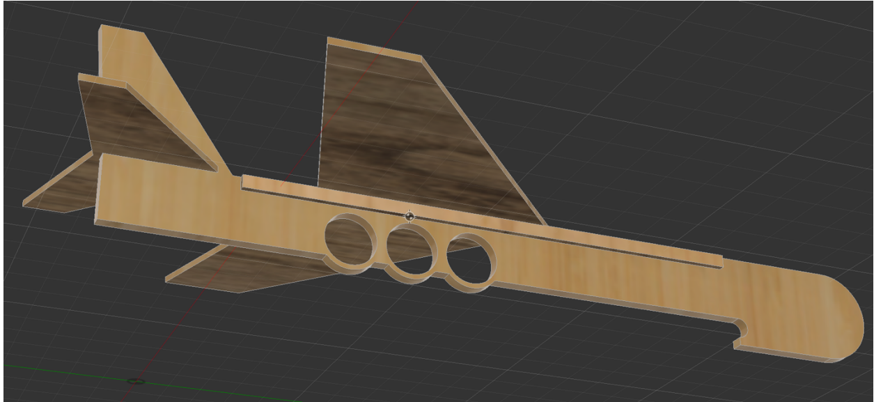
Figure 1: Merged assembly with associated wood properties. Fuselage 1/8" thick basswood; delta wing and stabilizers 1/16" basswood.
