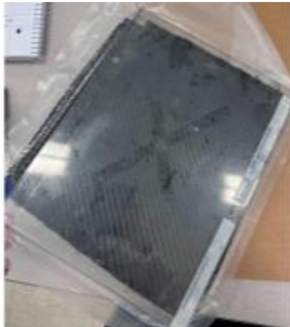
Figure 2. Laminated composite pressed in a vacuum bag to prevent voids during curing
