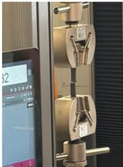
Figure 4. Instron tensile setup for tensile testing.
