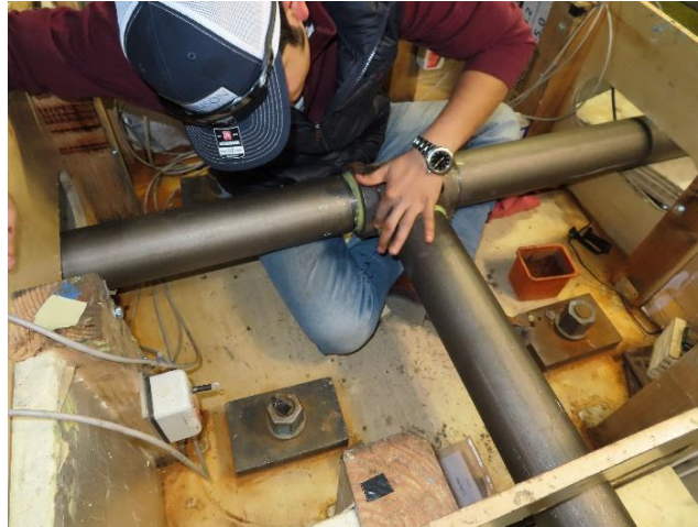
Figure 2. Allen Rivas Installing a Strain Gauge on a Specimen
